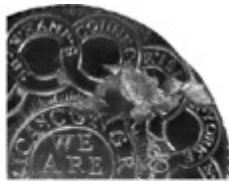
A defective planchet showing what is referred to as a “blow hole.”
