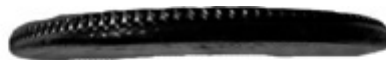
Edge view of a partial collar strike on a Nevada state quarter.
