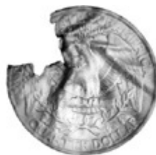
Washington quarter missing clad layer (the nickel layer itself).
